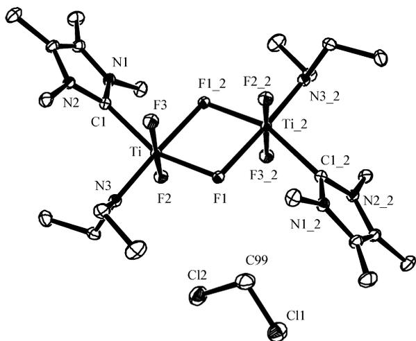
**Figure 3.** X-ray crystal structure of  $[\{\text{TiF}_2(\text{L}^{\text{Me}})(\text{NEt}_2)\}_2(\mu\text{-F})_2] \cdot 2\text{CH}_2\text{Cl}_2$ . Ellipsoids represent 50% probability levels. Hydrogen atoms and one  $\text{CH}_2\text{Cl}_2$  are omitted for clarity.
